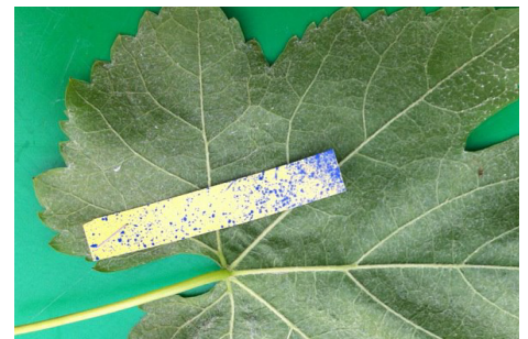
The Bertolini Sprayer achieved excellent coverage on the undersides of leaves in the middle of the canopy
